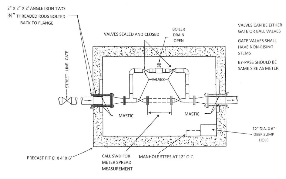
TYPICAL METER PIT REQUIREMENTS FOR 1 1/2" & 2" METER INSTALLATION
