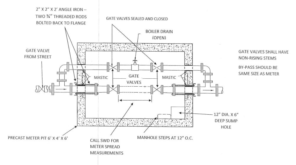
TYPICAL METER PIT REQUIREMENTS FOR 3" AND 4" METER INSTALLATION
